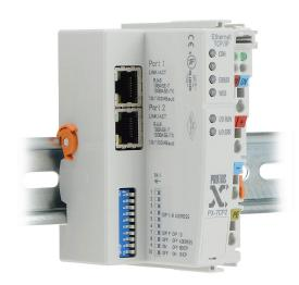
Protos X bus coupler, 24 VDC, (2) Ethernet (RJ45) port(s), Modbus TCP, 10/100 Mbps. For use with Protos X I/O systems.
