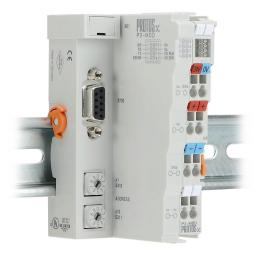
Protos X bus coupler, 24 VDC, (1) RS-485 (9-pin D-sub) port(s), Modbus RTU and ASCII, up to 38.4k baud. For use with Protos X I/ O systems.
