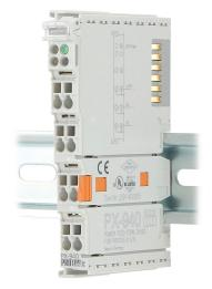
Protos X power feed terminal, 24 VDC. For use with Protos X I/O systems. Introduces power into I/O terminals power bus or switches from one voltage source to another for power flow to the right.
