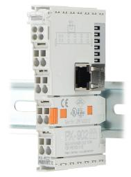
Protos X bus expansion end terminal, (1) Ethernet (RJ45) port(s). For use with Protos X I/O systems. Requires Ethernet (RJ45) cable. Used only with bus coupler, replaces PX-901 bus end terminal.
