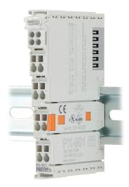
Protos X bus end terminal, for use with Protos X I/O systems. Installs at the right end of the terminal assembly. Required for proper communications between the I/O terminals and the bus coupler.
