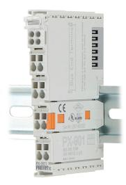
Protos X bus end terminal, for use with Protos X I/O systems. Installs at the right end of the terminal assembly. Required for proper communications between the I/O terminals and the bus coupler.
