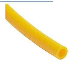
NITRA pneumatic tubing, ether-based polyurethane, yellow, 5/16in (8mm) outside diameter, 5mm inside diameter, 100ft package.
