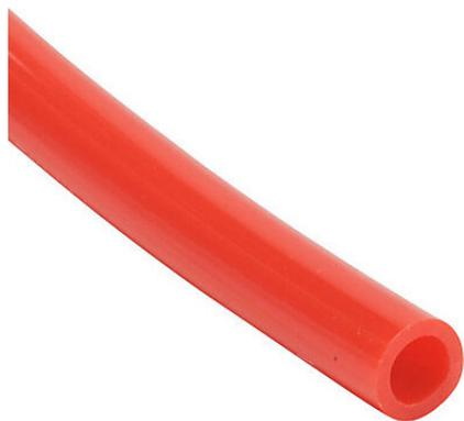
NITRA pneumatic tubing, ether-based polyurethane, red, 5/16in (8mm) outside diameter, 5mm inside diameter, 100ft package.
