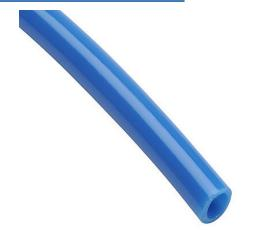
NITRA pneumatic tubing, ether-based polyurethane, blue, 5/16in (8mm) outside diameter, 5mm inside diameter, 500ft reel.
