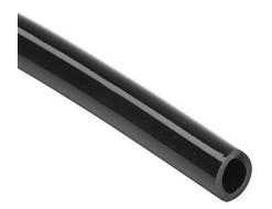
NITRA pneumatic tubing, ether-based polyurethane, black, 5/16in (8mm) outside diameter, 5mm inside diameter, 100ft package.
