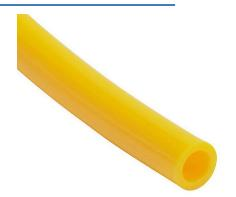
NITRA pneumatic tubing, ether-based polyurethane, yellow, 6mm outside diameter, 5/32in (4mm) inside diameter, 500ft reel.
