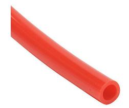
NITRA pneumatic tubing, ether-based polyurethane, red, 6mm outside diameter, 5/32in (4mm) inside diameter, 500ft reel.
