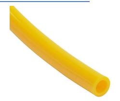
NITRA pneumatic tubing, ether-based polyurethane, yellow, 5/32in (4mm) outside diameter, 0.093in inside diameter, 100ft package.
