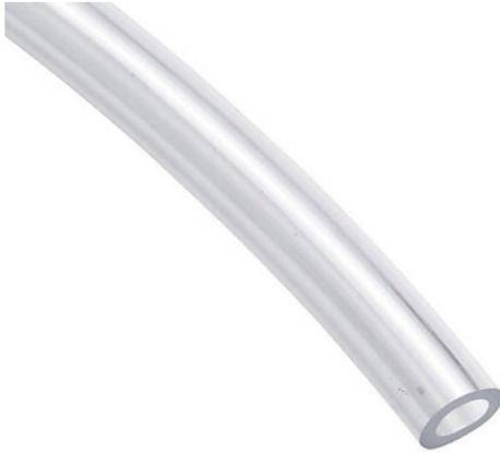
NITRA pneumatic tubing, ether-based polyurethane, clear, 5/32in (4mm) outside diameter, 0.093in inside diameter, 500ft reel.
