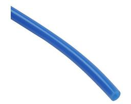
NITRA pneumatic tubing, ether-based polyurethane, blue, 5/32in (4mm) outside diameter, 0.093in inside diameter, 500ft reel.
