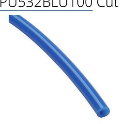
NITRA pneumatic tubing, ether-based polyurethane, blue, 5/32in (4mm) outside diameter, 0.093in inside diameter, 100ft package.
