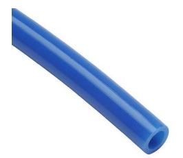
NITRA pneumatic tubing, ether-based polyurethane, blue, 3/8in outside diameter, 0.250in inside diameter, 100ft package.
