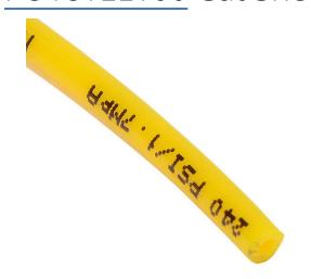
NITRA pneumatic tubing, ether-based polyurethane, yellow, 1/8in outside diameter, 0.062in inside diameter, 100ft package.
