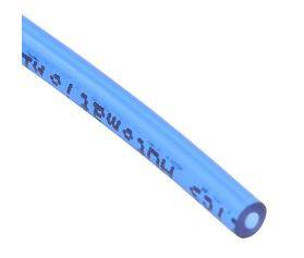
NITRA pneumatic tubing, ether-based polyurethane, clear blue, 1/8in outside diameter, 0.062in inside diameter, 100ft package.
