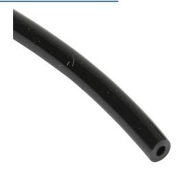
NITRA pneumatic tubing, ether-based polyurethane, black, 1/8in outside diameter, 0.062in inside diameter, 500ft reel.
