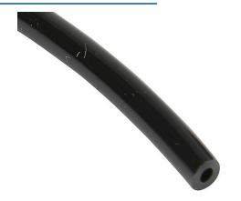
NITRA pneumatic tubing, ether-based polyurethane, black, 1/8in outside diameter, 0.062in inside diameter, 100ft package.
