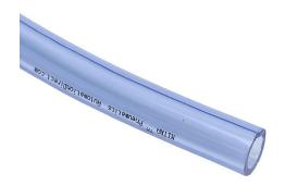
NITRA pneumatic tubing, ether-based polyurethane, clear blue, 16mm outside diameter, 11mm inside diameter, 100ft package.
