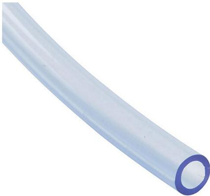
NITRA pneumatic tubing, ether-based polyurethane, clear blue, 1/4in outside diameter, 0.156in inside diameter, 100ft package.
