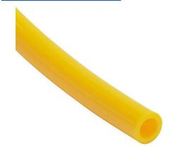
NITRA pneumatic tubing, ether-based polyurethane, yellow, 1/2in outside diameter, 0.328in inside diameter, 100ft package.
