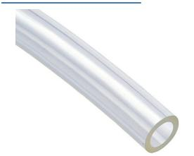
NITRA pneumatic tubing, ether-based polyurethane, clear, 10mm outside diameter, 6.5mm inside diameter, 500ft reel.
