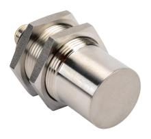
ProSense inductive proximity sensor, tubular, 30mm diameter x 65mm body, stainless steel housing, PNP, N.O. output, 25mm sensing distance, non-flush, 100 Hz switching frequency, IP65 IP66 IP67 IP68 IP69K, 4-pin M12 quick-disconnect.
