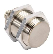
ProSense inductive proximity sensor, tubular, 30mm diameter x 50mm body, stainless steel housing, PNP, N.O. output, 15mm sensing distance, flush, 50 Hz switching frequency, IP65 IP66 IP67 IP68 IP69K, 4-pin M12 quick-disconnect.
