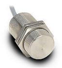
AutomationDirect inductive proximity sensor, tubular, 30mm diameter x 50mm body, stainless steel housing, PNP, N.O. output, 20mm sensing distance, flush, 100 Hz switching frequency, IP68, pigtail.
