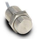
AutomationDirect inductive proximity sensor, tubular, 30mm diameter x 50mm body, stainless steel housing, NPN, N.O. output, 20mm sensing distance, flush, 100 Hz switching frequency, IP68, pigtail.
