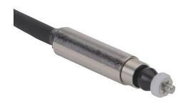
Metrol limit switch, precision touch, 5mm diameter, smooth, 25mm length, 2mm radius head, stainless steel, 1.5mm plunger, 0.8N contact force, N.C. contact(s), 6.5ft/2m cable length, pigtail.
