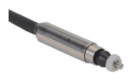
Metrol limit switch, precision touch, 5mm diameter, smooth, 25mm length, 2mm radius head, stainless steel, 1.5mm plunger, 0.8N contact force, (1) N.C. contact(s), 6.5ft/2m cable length, pigtail.
