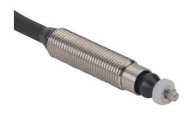
Metrol limit switch, precision touch, 5mm diameter, threaded, 0.5mm pitch, 25mm length, 2mm radius head, stainless steel, 1.5mm plunger, 0.8N contact force, (1) N.C. contact(s), 6.5ft/2m cable length, pigtail.
