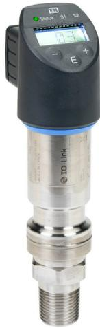
Endress+Hauser Ceraphant digital pressure sensor, 0 to 6000 psig range, Output: 4-20 mA, Output 2: switch PNP, N.O./N.C. selectable or IO-Link, 1/2in male NPT or 1/4in female NPT process connection.
