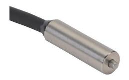
Metrol limit switch, precision touch, 5mm diameter, smooth, 18.5mm length, 2mm radius head, stainless steel, 1.5mm plunger, 0.5N contact force, (1) N.C. contact(s), 6.5ft/2m cable length, pigtail.
