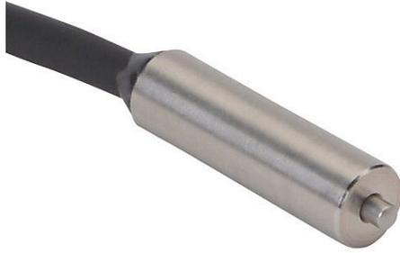
Metrol limit switch, precision touch, 5mm diameter, smooth, 18.5mm length, 2mm radius head, stainless steel, 1.5mm plunger, 0.5N contact force, (1) N.C. contact(s), 6.5ft/2m cable length, pigtail.
