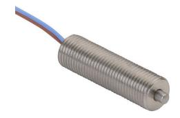
Metrol limit switch, precision touch, 5mm diameter, threaded, 0.5mm pitch, 18.5mm length, 2mm radius head, stainless steel, 1.5mm plunger, 0.5N contact force, (1) N.C. contact(s), 1.6ft/0.5m cable length, core wire.
