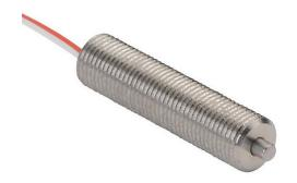
Metrol limit switch, precision touch, 5mm diameter, threaded, 0.5mm pitch, 21.5mm length, 2mm radius head, stainless steel, 1.5mm plunger, 0.5N contact force, N.O. contact(s), 1.6ft/0.5m cable length, core wire.
