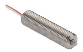
Metrol limit switch, precision touch, 5mm diameter, threaded, 0.5mm pitch, 21.5mm length, 2mm radius head, stainless steel, 1.5mm plunger, 0.5N contact force, (1) N.O. contact(s), 1.6ft/0.5m cable length, core wire.
