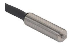
Metrol limit switch, precision touch, 5mm diameter, threaded, 0.5mm pitch, 18.5mm length, 2mm radius head, stainless steel, 1.5mm plunger, 0.5N contact force, N.C. contact(s), 6.5ft/2m cable length, pigtail.
