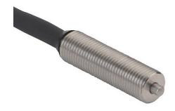
Metrol limit switch, precision touch, 5mm diameter, threaded, 0.5mm pitch, 18.5mm length, 2mm radius head, stainless steel, 1.5mm plunger, 0.5N contact force, (1) N.C. contact(s), 6.5ft/2m cable length, pigtail.
