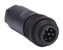
Field wireable connector, PG16 thread nut 7-pin male axial, accepts cable diameter size 12-14mm, 22 - 16 AWG, screw terminal connection, IP67.
