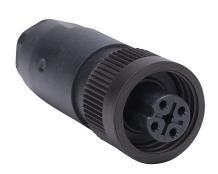
Field wireable connector, PG13.5 thread nut 4-pin female axial, accepts cable diameter size 10-12mm, 20 - 14 AWG, screw terminal connection, IP67.
