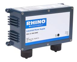
RHINO TOUGH PSX series switching power supply, 12 VDC @ 8A/96W (adjustable), 120/240 VAC or 85-375 VDC nominal input, 1-phase, encapsulated, die-cast aluminum housing, chassis mount, screw connectors, hazardous location rated.
