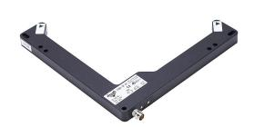
AutomationDirect photoelectric fork sensor, L-frame, die-cast zinc housing, through-beam, visible red, 0-160mm sensing distance, 10-30 VDC operating voltage, selectable light-on/dark-on, PNP, 3-pin M8 quick-disconnect.
