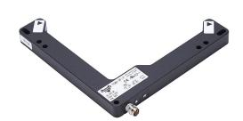
AutomationDirect photoelectric fork sensor, L-frame, die-cast zinc housing, through-beam, visible red light emission, 0-130mm sensing distance, 10-30 VDC operating voltage, selectable light-on/dark-on, PNP, 3-pin M8 quick-disconnect.
