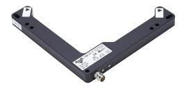
AutomationDirect photoelectric fork sensor, L-frame, die-cast zinc housing, through-beam, visible red, 0-130mm sensing distance, 10-30 VDC operating voltage, selectable light-on/dark-on, PNP, 3-pin M8 quick-disconnect.
