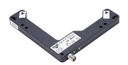
AutomationDirect photoelectric fork sensor, L-frame, die-cast zinc housing, through-beam, visible red, 0-100mm sensing distance, 10-30 VDC operating voltage, selectable light-on/dark-on, PNP, 3-pin M8 quick-disconnect.
