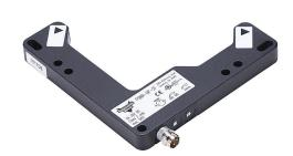
AutomationDirect photoelectric fork sensor, L-frame, die-cast zinc housing, through-beam, visible red, 0-80mm sensing distance, 10-30 VDC operating voltage, selectable light-on/dark-on, PNP, 3-pin M8 quick-disconnect.
