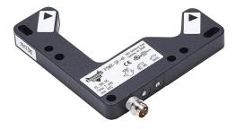
AutomationDirect photoelectric fork sensor, L-frame, die-cast zinc housing, through-beam, visible red, 0-60mm sensing distance, 10-30 VDC operating voltage, selectable light-on/dark-on, PNP, 3-pin M8 quick-disconnect.
