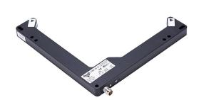
AutomationDirect photoelectric fork sensor, L-frame, die-cast zinc housing, through-beam, visible red, 0-160mm sensing distance, 10-30 VDC operating voltage, selectable light-on/dark-on, NPN, 3-pin M8 quick-disconnect.
