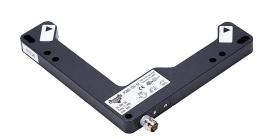
AutomationDirect photoelectric fork sensor, L-frame, die-cast zinc housing, through-beam, visible red, 0-100mm sensing distance, 10-30 VDC operating voltage, selectable light-on/dark-on, NPN, 3-pin M8 quick-disconnect.
