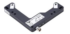
AutomationDirect photoelectric fork sensor, L-frame, die-cast zinc housing, through-beam, visible red, 0-80mm sensing distance, 10-30 VDC operating voltage, selectable light-on/dark-on, NPN, 3-pin M8 quick-disconnect.
