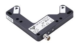
AutomationDirect photoelectric fork sensor, L-frame, die-cast zinc housing, through-beam, visible red, 0-60mm sensing distance, 10-30 VDC operating voltage, selectable light-on/dark-on, NPN, 3-pin M8 quick-disconnect.
