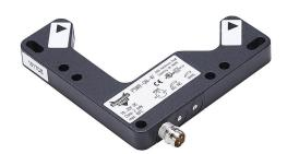
AutomationDirect photoelectric fork sensor, L-frame, die-cast zinc housing, through-beam, visible red light emission, 0-60mm sensing distance, 10-30 VDC operating voltage, selectable light-on/dark-on, NPN, 3-pin M8 quick-disconnect.
