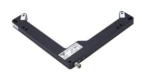
AutomationDirect photoelectric fork sensor, L-frame, die-cast zinc housing, through-beam, infrared, 0-160mm sensing distance, 10-30 VDC operating voltage, selectable light-on/dark-on, PNP, 3-pin M8 quick-disconnect.
