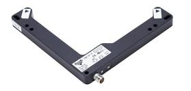
AutomationDirect photoelectric fork sensor, L-frame, die-cast zinc housing, through-beam, infrared light emission, 0-130mm sensing distance, 10-30 VDC operating voltage, selectable lighton/dark-on, PNP, 3-pin M8 quick-disconnect.
