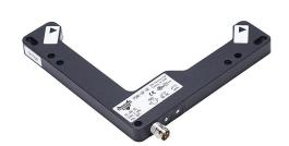
AutomationDirect photoelectric fork sensor, L-frame, die-cast zinc housing, through-beam, infrared, 0-100mm sensing distance, 10-30 VDC operating voltage, selectable light-on/dark-on, PNP, 3-pin M8 quick-disconnect.
